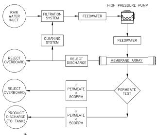
Figure 3.2: Simplified Schematic of an RO System.
