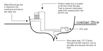
Figure 2.1: Recommended installation BELOW waterline.
