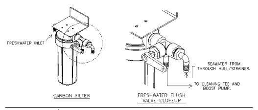
Figure 2.2: Carbon Filter with Freshwater Flush Valve – Isometric Views.
