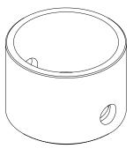
Fig. 6: Seal Retainer
