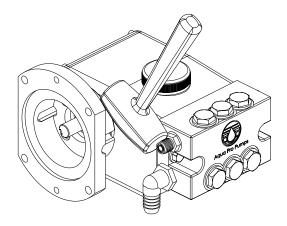
Fig. 2: Manifold Assembly Removal
