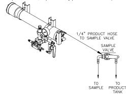
Figure 2.5: Little Wonder MODULAR Sample Valve Connection.
