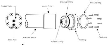
Figure 6.1 - Pressure Vessel End Plug Assembly Callout.
