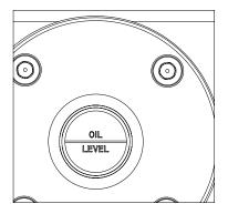
Fig. 1: Oil Level Sight Glass Detail.
